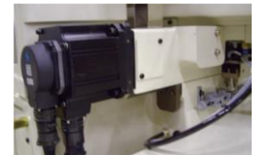
Servo Motor drive for longitudinal feed
