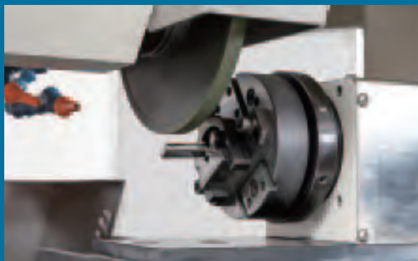
Round Punch & Elliptical Punch can be done by NC Index device
