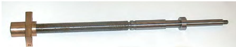
FINE CROSS FEED SCREW & BUSHING
